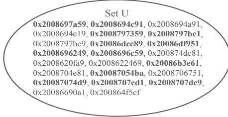
Figure 4: Set U shows the set of all addresses that flipped across 8 attempts to restore the data and hammering the same chunk from Figure 3. The boldfaced addresses are addresses that flipped more than once across the 8 attempts.
